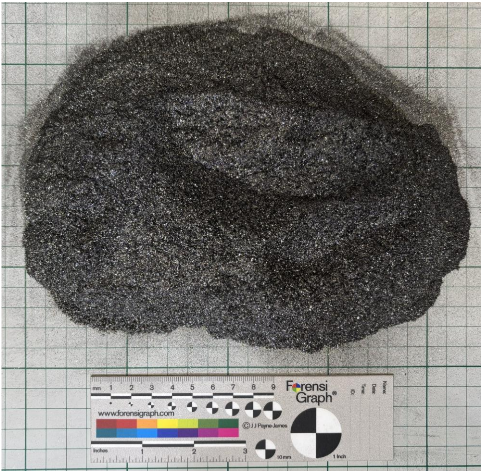
Figure II-15. Photograph of natural state graphite concentrate.
