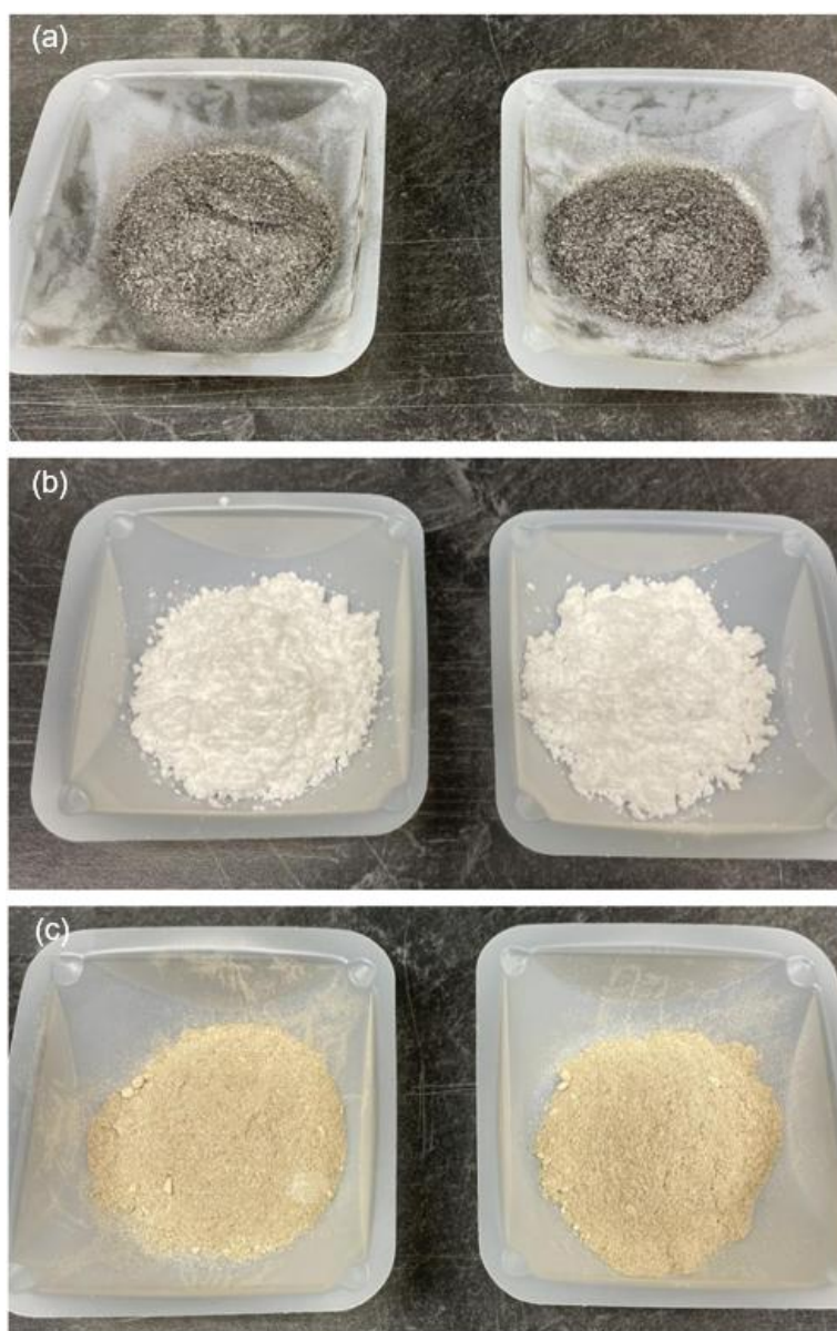
Figure 16. Photographs of a selection of host materials dispatched to Microtrace for testing with Microtrace's Molecular™ Taggant System. (a) Graphite concentrate, (b) lithium carbonate, and (c) lithium ore. The host material on the left of each image is untagged, while the host material on the right is tagged.
