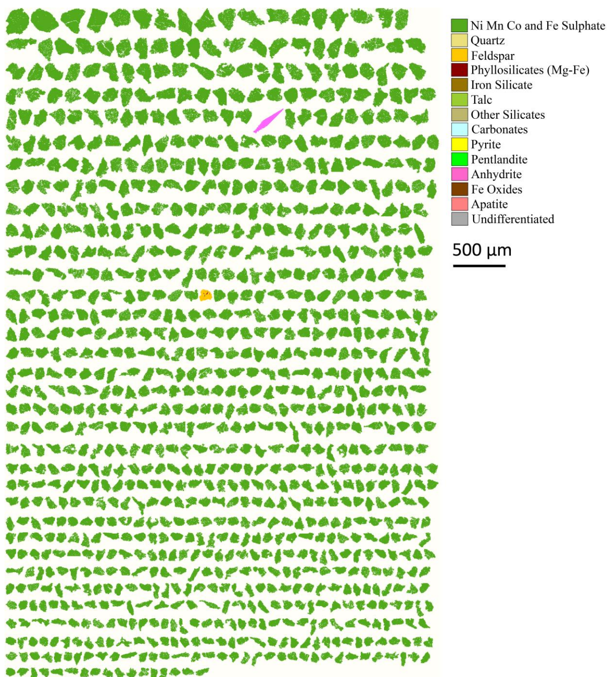
Figure II-23. Mixed hydroxide precipitate image arranged by area (subsample 1).
