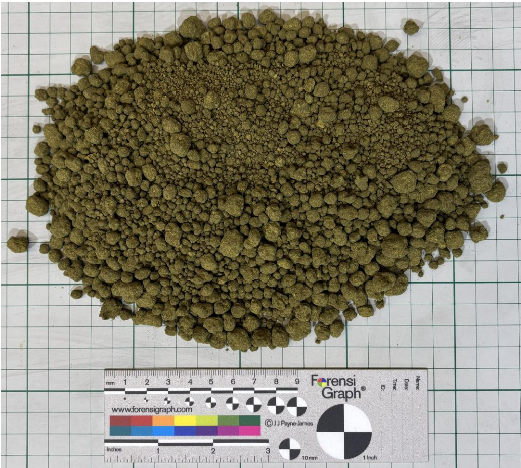
Figure II-20. Photograph of natural state mixed hydroxide precipitate.
