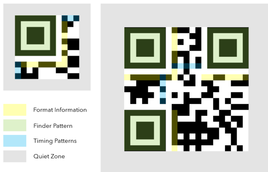
Figure 2. Comparison of an M1 micro QR code (left) and a Version 1 QR code (right). The QR codes yield the numeric encoding "12345". Figure adapted from Karrach et al. (2020) and Scandit (2026).
