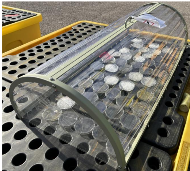
Figure 12. Photooxidative ageing samples mid-test.
