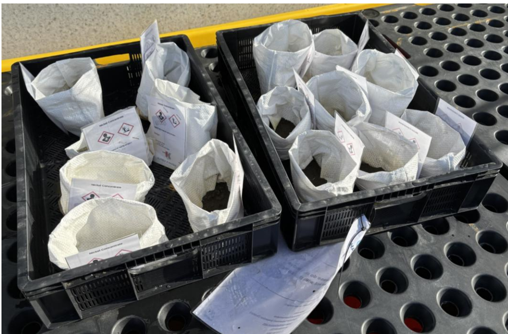
Figure 11. Natural ageing samples mid-test.
