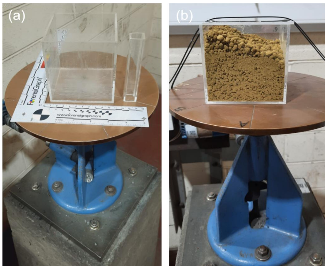
Figure 10. Flow Table Test apparatus and poly(methyl methacrylate) (PMMA) cube. (a) Apparatus used for the test including PMMA cube and cuboid spear. (b) Sealed PMMA cube for the Modified Flow Table Test.
