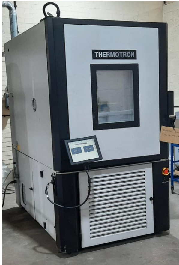
Figure 13. Thermotron SE1000-3-3 Environmental Chamber.
